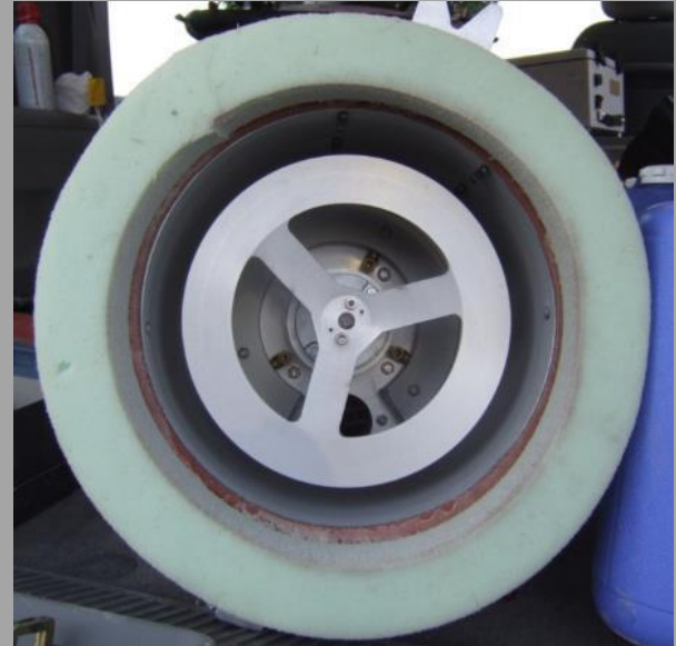
Figure 2: PI-SWERL fan. Image by Desert Research Institute
