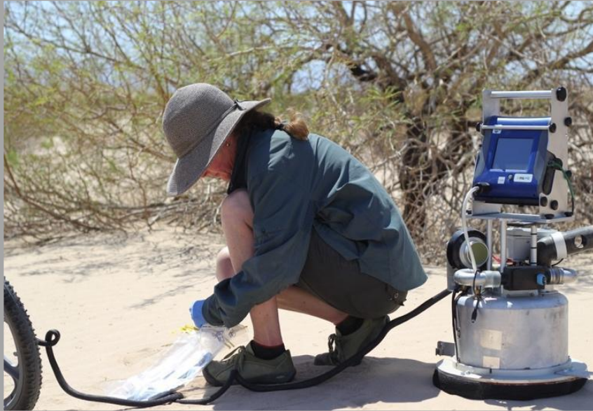
Figure 3: Karen Foley collecting PI-SWERL (portable wind shear chamber) samples in the Sonoran Desert.
