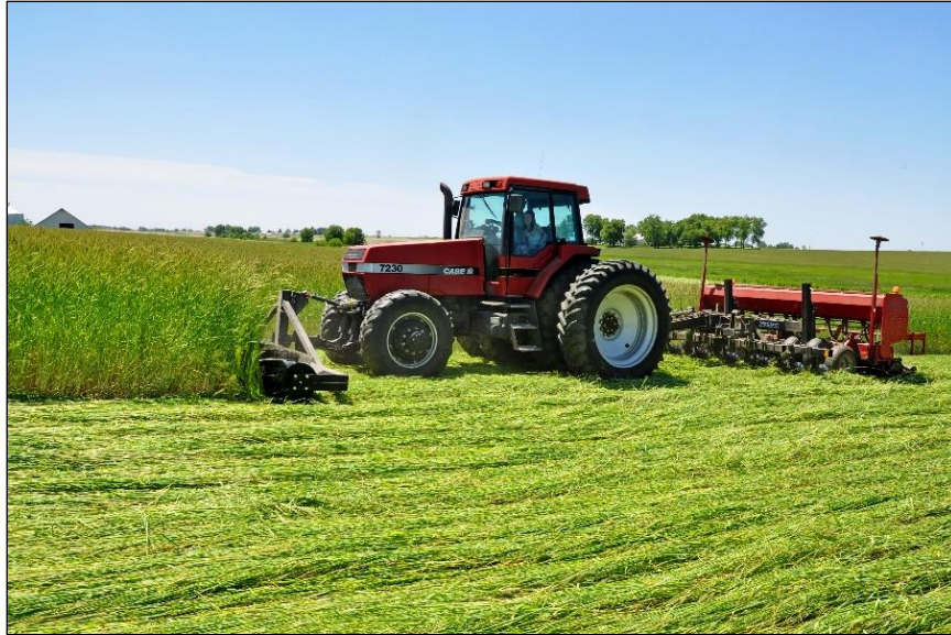
Figure 6-17. Here Levi crimps his cereal rye cover crop and plants soybeans directly in the matted cover crop. Photo: Jason Johnson, USDA NRCS, March 2017.
