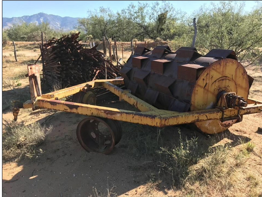
Figure 7-25. The range imprinter can be utilized to restore degraded rangeland as a method of Grazing Land Mechanical Treatment (548). The imprinter creates an uneven surface to interrupt sheet flow and encourage additional moisture to enter the soil. The imprinter does not perform well in hard, compacted soils, where thick desert pavement exists or where large rock fragments exist. Photo: USDA-NRCS Gilbert Two Two.
