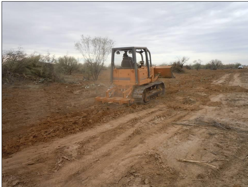
Figure 7-28. Grazing Land Mechanical Treatment (548) practiced post-Brush Management (314) treatment and prior to Range Planting (550). In this case Grazing Land Mechanical Treatment is utilized to break up compaction and surface seal prior to seed planting to improve planting success. Photo: USDA NRCS, Gilbert Two Two.
