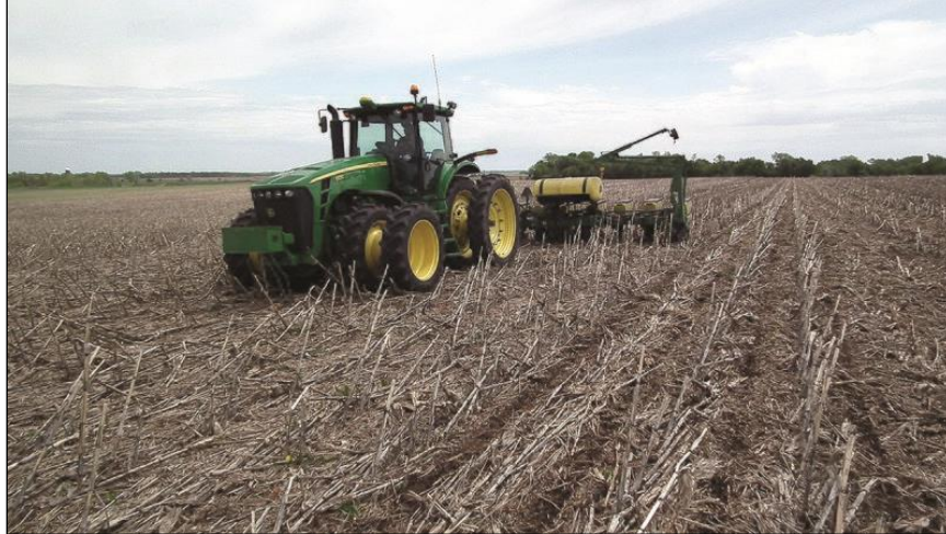
Figure 6-8. Residue Management, No-Till (329). Direct seeding into prior crop's residue, with fertilizer application. Photo: Eric Barsness, USDA NRCS South Dakota, June 2013.
